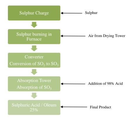
Sulphur is melted in Sulphur pit. Molten Sulphur is burnt in Sulphur furnace in the presence of air. Sulphur dioxide  $(SO_2)$  gas goes to the converter where it is converted in Sulphur trioxide  $(SO_3)$  in presence of vanadium catalyst.  $SO_3$  is then absorbed in absorption tower where 98% Sulphuric acid is circulated. This gives Sulphuic Acid or Oleum 25%.
